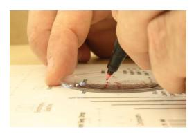
We will pre-mark DST engravings for you. All DST lenses must have the reference marks recreated on the <u>back surface</u> of the lens, where the engravings are located.
